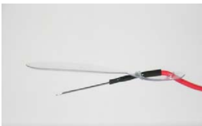
Fig 1. Low-cost prototype of IONM needle electrode incorporating a safety flap
